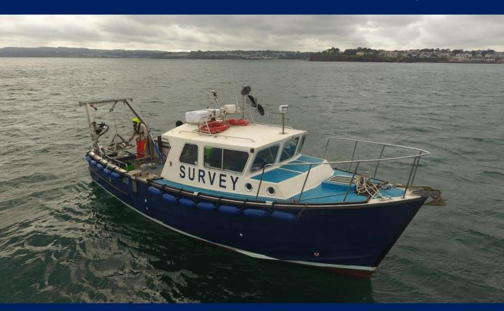
'Seren Las' is a 10 m MCA Category 2 coded survey and dive support vessel refitted in 2017 to enhance its marine survey capabilities. With ample deck space and a purpose-designed hydraulic gantry and winch it is an ideal platform for a variety of survey requirements.
